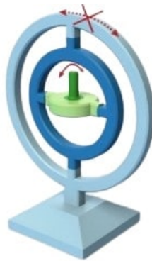
Figure 2.7 Illustration of gimbal lock, the inner axis (dark green) cannot be rotated in the direction of the dotted arrows [Haslwanter, 2018]
